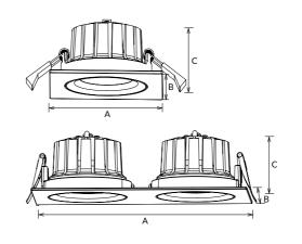
NC76B is a square COB LED downlight with aluminum die-casting housing. It could be tilted 25 degree, 15°/24°/36°/60°beam angle for selection. Dim to warm(2000K~3000K) and ficker free external driver are available.
