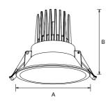
NC103B fxed downlight adopts high effciency SMD LED chips, PMMA lens and ADC12 aluminum heatsink. Deep cone design creates low UGR. External driver is exchangeable through quick connector among non-dimmable driver, Triac dimmable, 0-10V and DALI dimmable drivers.
