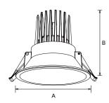
NC103 fxed downlight adopts brand CREE COB, refector and ADC12 aluminum heatsink. Deep cone design creates low UGR. External driver is exchangeable through quick connector among non-dimmable driver, Triac dimmable, 0-10V and DALI dimmable drivers.
